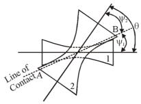
**Crossed helical gears**: The use of crossed-helical gears or spiral gears is limited to light loads. Therse gears are used to drive feed mechanism on machine tools, camshafts and oil pumps in l.C. engine.
