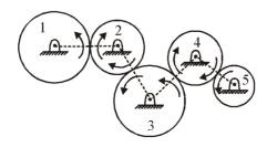
A series of gears, capable of receiving and transmitting motion from one gear axes remain fixed relative to the frame and each gear is on separates shaft.
