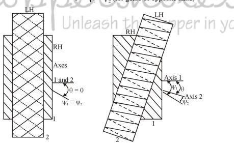
Angle between shafts,  $\theta = \psi_1 + \psi_2$  for gears of same hand  $\theta = \psi_1 - \psi_2$ . for gears of opposite hand. for  $\psi_1 - \psi_2$ ,  $\theta = 0$ , a case of helical gears joining parallel shafts.
