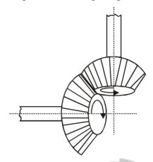
**Spiral bevel Gears**: When the teeth of a bevel gear are inclined at angle to the face of the bevel, they are known as spiral bevel or helical bevels.
