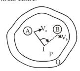
Let a plane body 'P' having non-linear motion relative to another plane body Q. At any instant, the linear velocities of the point 'A' and 'B' on the body 'P' are ' $V_a$ ' and ' $V_b$ ' respectively.
