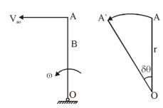
as  $\delta t \rightarrow 0$ , AA' will be perpendicular to OA. Thus the velocity of A is  $\omega r$  and is perpendicular to OA.
