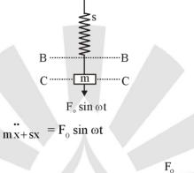
$$x = x\sin(\omega_n t + \phi) + \frac{\frac{F_o}{s}}{1 - \left(\frac{\omega}{\omega_n}\right)^2} \sin\omega t$$
