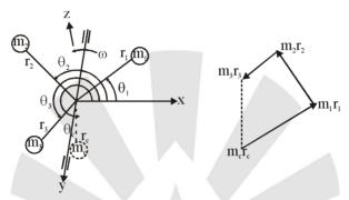
The rotor is said to be statically balanced. If vector sum of centrifugal force (F) is zero.
