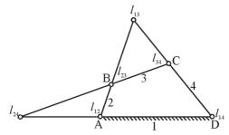
It is used to find angular velocity of a link if angular velocity of another link is known.
