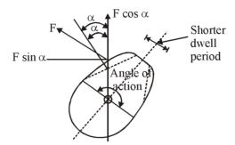
In order to reduce the lateral pressure of  $F \sin \alpha$ ,  $\alpha$  has to be decreased which means making the surface more convex and longer. This results in reduced velocity of the follower and more time for the same rise. Minimum value of  $\alpha$  cannot be reduced from a certain value.
