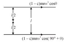
Unbalanced primary forces along the lines of stroke the separated by a distance *l* apart and thus constitute a couple. This tends to make the leading wheels sway from side to side.
