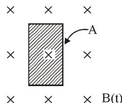
**Case-II :** Iron piece is stationary but B is changing w.r.t time (e.g. transformers), so  $\phi = BA$  is changing w.r.t time.
