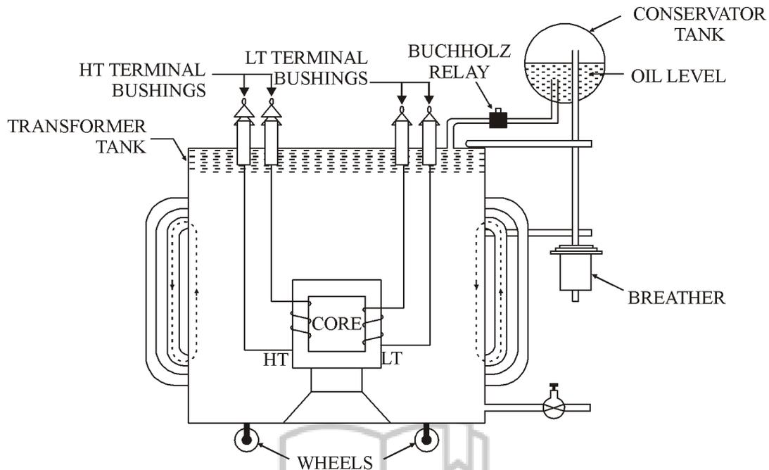
1. **Core Construction:** A transformer core is the steel system which forms the magnetic circuit with all parts pertaining to its construction. Those parts of the magnetic circuit, which carry the transformer windings are called the limbs or legs, and those parts which connect the legs and serve for closing the magnetic circuit are termed yokes.
