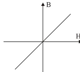
For linear magnetic circuit
