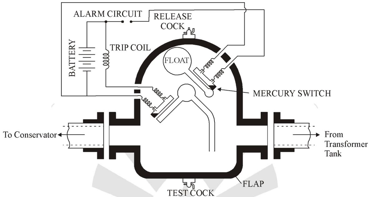
*Fig. Gas operated relay*
