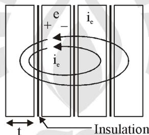
As resistance is introduced in the path of eddy currents so resistance  $R_e$  increases & hence power loss decreases.
