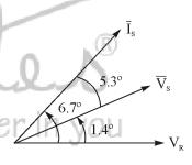
$\overline{I}_{\!_{S}}$  leads  $\,\overline{V}_{\!_{S}}\,$  by  $5.3^o$
