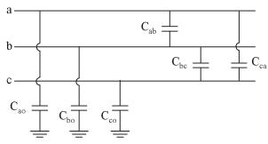
$C_{ao},\,C_{bo},\,C_{co}\Rightarrow Capacitance$  between line and ground
