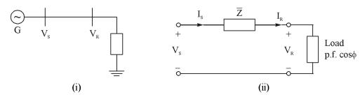
At lagging power factor  $cos\varphi,$  receiving end current  $I_R$  lags  $V_R$  by angle  $\varphi.$
