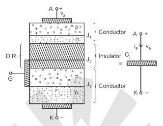
Due to higher charging current, large number of charge carriers crosses the  $J_2$  which may create breakdown of D.R. & SCR may turn-ON even without gate signal, it is said to be  $\frac{dv_a}{dt}$  triggering.
