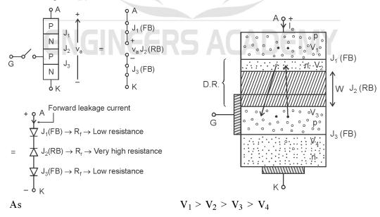
So  $J_2$  is reverse biased & depletion region exists there, most of the width of D.R. is lying in n-layer as it is very lightly doped in comparison to inner p-layer.
