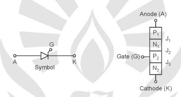
Approximate level of doping of layers outer layers  $P_1$  &  $N_2$  is  $10^{19}/\text{cm}^3$  i.e. high doped, inner p-layer i.e.  $P_2$  is  $10^{17}/\text{cm}^3$  & inner N-layer i.e.  $N_1$  has  $10^{13}$  to  $5 \times 10^{14}$  / cm<sup>3</sup> (i.e. very lightly doped).
