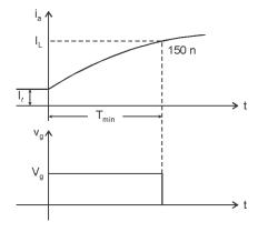
At t = 0, SCR is fired,  $i_a$  starts increasing from leakage current  $I_l$  so number of charge carriers crossing  $J_2$  increases.
