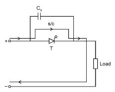
As thyristor acts as open circuited (forward blocking mode) &  $C_s$  as short circuited so transient is bypassed from the thyristor thus protecting the thyristor. Once transient/noise is over  $C_s$  gets charged say upto voltage  $V_c$ . Whenever T is fired  $C_s$  will discharge through T (i.e. forward Conduction mode & low resistance path).
