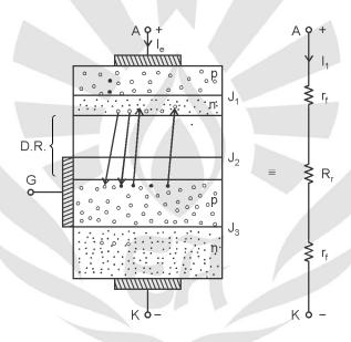
In forward blocking mode, the forward leakage current  $I_l$  is flowing due to minority charge carriers. As reverse biased  $J_2$  offers high resistance  $R_r (\cong M\Omega)$  so power loss  $I_l^2 R_r$  occurs mainly across  $J_2$ . To avoid thermal runaway (i.e. temperature triggering) the heat developed across  $J_2$  is continuously removed using  $A_1$  heat sink.
