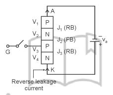
As K is at higher potential than A, the voltage decreases progressively from K to A
