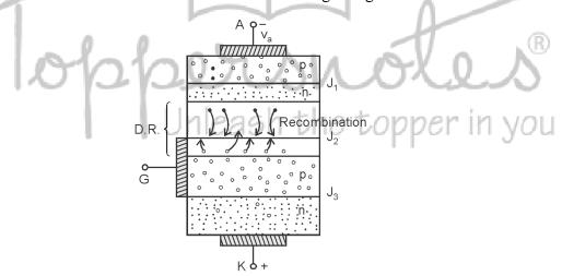
So to remove excess charge carriers around  $J_2$  it should be reverse biased for short duration. The excess charge carriers will be lost by recombination. So to commutate (or to turn-off) SCR  $i_a$  should be reduced below  $I_H$  & then it should be kept reversed for time  $t_q$ .
