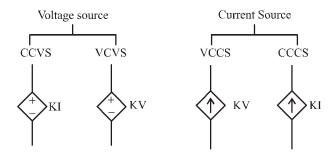
Inherently the controlled sources are also non-linear in nature, since the voltage and current relationship is non-linear. But the linearity of the controlled source is defined w.r.t. controlling independent variable. If they are linear, then the sources are said to be linear, otherwise non-linear.
