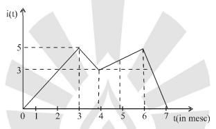
Solution: The area of under curve i(t) and t gives stored charge
