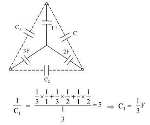
$$\frac{1}{C_2} = \frac{\frac{1}{3} \times \frac{1}{2} + \frac{1}{1} \times \frac{1}{2} + \frac{1}{1} \times \frac{1}{3}}{\frac{1}{1}} = 1$$
