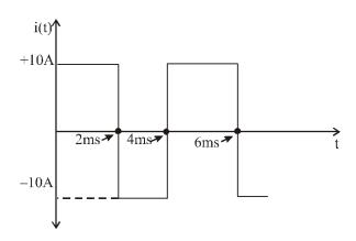
$$\begin{split} I_{rms}^2 &= \frac{1}{4 \times 10^{-3}} \bigg[ \int_0^2 (10)^2 dt + \int_2^4 (-10)^2 dt \bigg] \\ &= \frac{1}{4 \times 10^{-3}} \big[ 100(2-0) + 100(4-2) \big] \times 10^{-3} \\ &= \frac{1}{4 \times 10^{-3}} \times 400 \times 10^{-3} = 100 \text{ A} \\ P_{rms} &= I_{rms}^2 \text{ R} = 100 \times 1 = 100 \text{ W} \\ P_{max} &= \big| I^2 \big|_{R} (10)^2 \times 1 \\ &= 100 \text{ W} \end{split}$$
