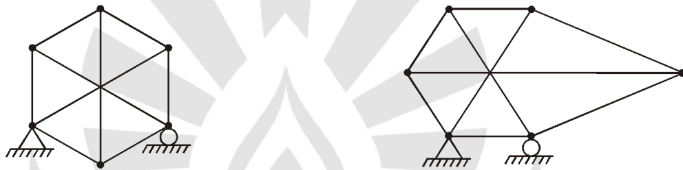
Fig. : (a) Unstable if all diagonals are of equal length
