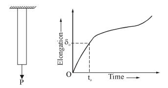
Consider a vertical bar loaded by constant force P. When load P is applied initially, the bar elongates by amount  $\delta_0$  during time  $t_0$ . Subsequent to time  $t_0$ , the load remains constant. However, due to creep, the bar elongatics even though load does not change. Creep is more at higher temperature than at ordinary temperature, i.e., creep is propotional to temperature.
