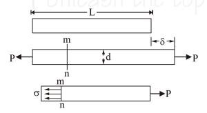
A section taken perpendicular to longitudinal axis of bar is cross-section. Considering free-body diagram, the tensile force P acts on right hand of free body at the other end is force representing the action of removed part of bar upon the part that remains. These forces are continuously distributed over the cross-section. The intensity of force (i.e. force per unit area) is called the stress and is denoted by, s
