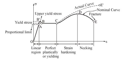
The typical stress strain diagram of mild steel is shown in figure. Here, the stress is nominal stress or engineering stress and strain is nominal strain or engineering strain.
