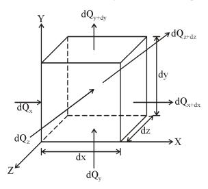
According to Fourier heat conduction law, the heat flowing into the left most face of the element in the X-direction.
