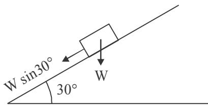
The component of gravity force parallel to inclined planes is
