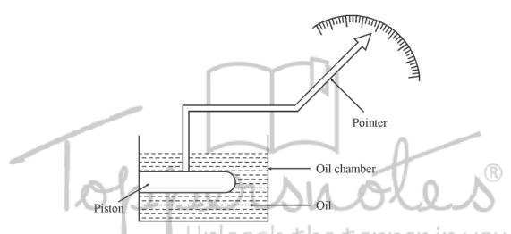
Example: The torque of an ammeter varies as the square of the current through it. If current of 10 Amp produces a deflection of 90°. What deflection will occur for a current of 6 amperes.
