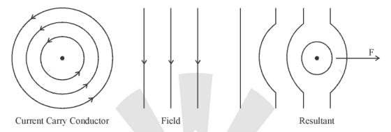
Current carrying conductor produced field. Dot shows upward current field is anti clockwise. If it is placed in magnetic field as shown then a force exerts as per left hand law or motor law.
