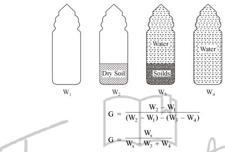
*Note*: Specific gravity values are generally reported at  $27^{\circ}$  C (in India) If  $T^{\circ}$  C is the test temperature then Sp. Gr. at  $27^{\circ}$  C is given by,
