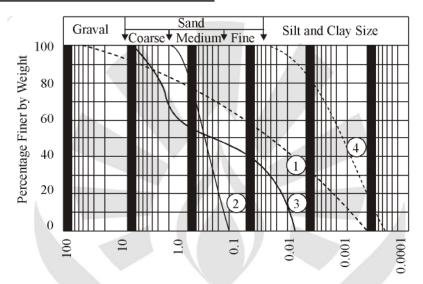
Curve 1: Well graded soil: good representation of grain sizes over a wide range and its gradation curve is smooth.
