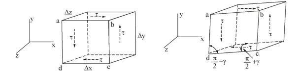
Considering force equilibrium total shear force on the top face is  $\tau \Delta x \Delta z$  and this force is balanced by equal and opposite force on bottom face. These two force form a couple having moment about z-axis of magnitude  $\tau \Delta x \Delta y$  Equilibrium of element requires this moment to be balanced by equal and opposite moment resulting from shear stress acting on side face of element.
