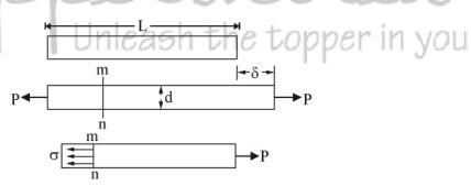
A section taken perpendicular to longitudinal axis of bar is cross-section. Considering free-body diagram, the tensile force P acts on right hand of free body at the other end is force representing the action of removed part of bar upon the part that remains. These forces are continuously distributed over the cross-section. The intensity of force (i.e. force per unit area) is called the stress and is denoted by, s
