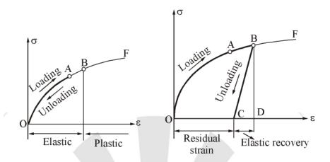
Suppose material is loaded and strain go from O to A. When load is removed, the material follow exactly the same curve back to origin O. This Property of material by which it returns to its original dimension during unloading is called elasticity and material is said to be elastic.
