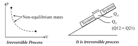
An irreversible process is usually represented by a dotted (or discontinuous) line joining the end states to indicate that the intermediate states are undetermined.
