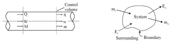
Heat, flow work and mass all can enter and leave the control volume
