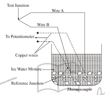
Due to seeback effect, a net e.m.f. is generated in circuit which depends on the difference in temperature between the hot and cold junction and is, therefore a thermometric property of the circuit the e.m.f. can be measured by a microvoltmeter to a high degree of accuracy.
