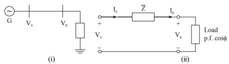
At lagging power factor  $cos\varphi,$  receiving end current  $I_R$  lags  $V_R$  by angle  $\varphi.$
