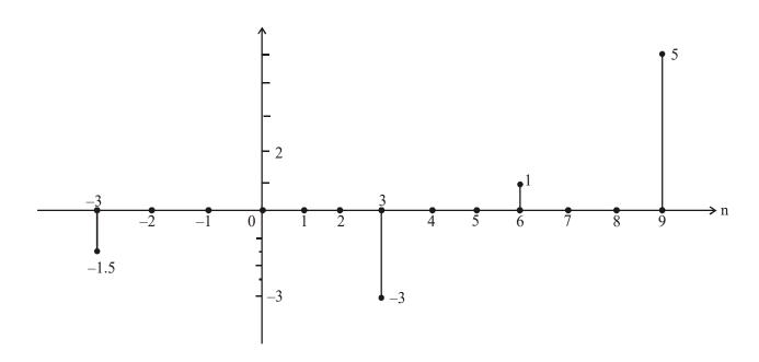
(iv) x(2n): It is the compression of discrete time signal: Compression of discrete time signal is called decimation. (loss of information)
