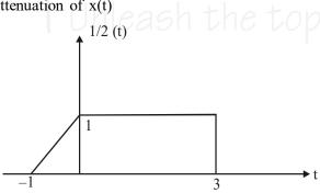
(v) -x(t) + 2: It is a composite operation, in the amplitude operation firstly obtain -x(t) then shift by +2 unit.
